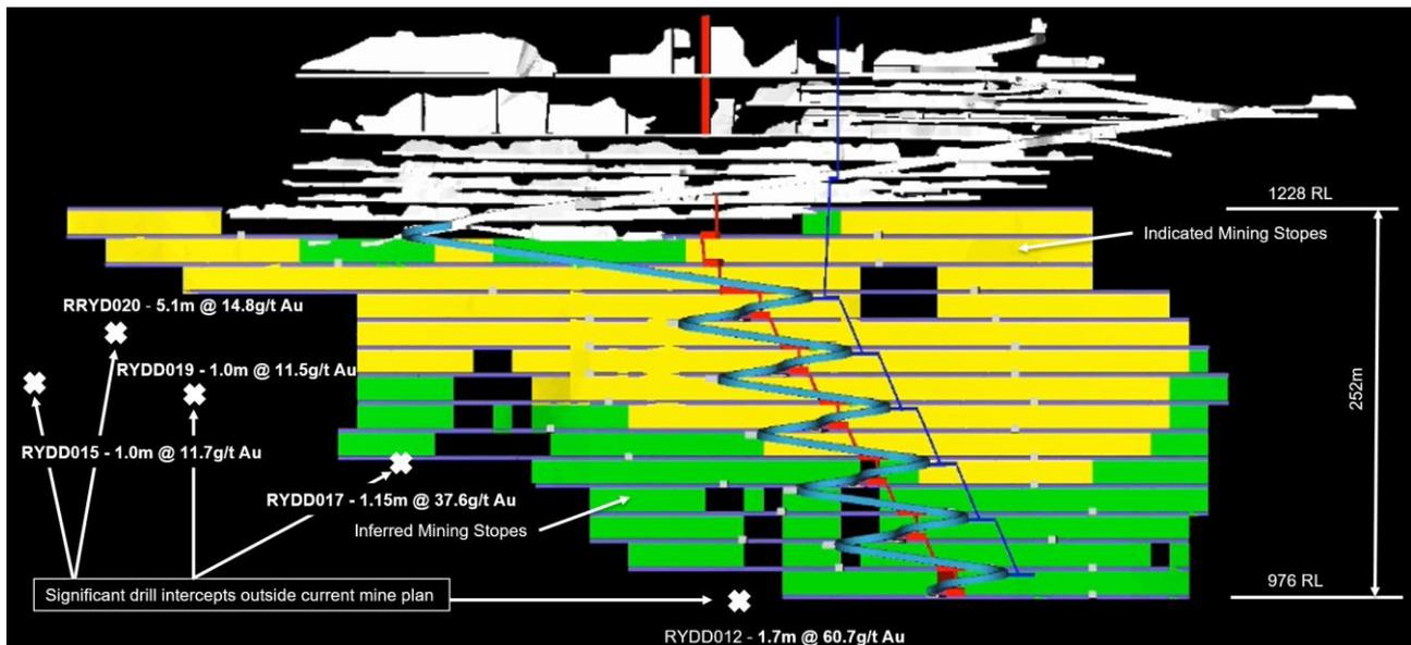
FIGURE 2 – ROTHSAY LONG PROJECTION SHOWING INDICATED AND INFERRED MINING STOPES AND PIERCE POINTS OF SIGNIFICANT INTERCEPTS OUTSIDE CURRENT MINE DESIGN
