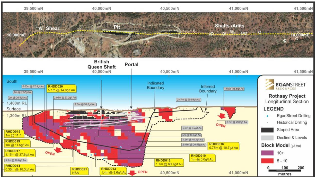
FIGURE 1 - "A" SHEAR LONG PROJECTION SHOWING DRILL INTERCEPTS OF RECENTLY COMPLETED DRILLING
