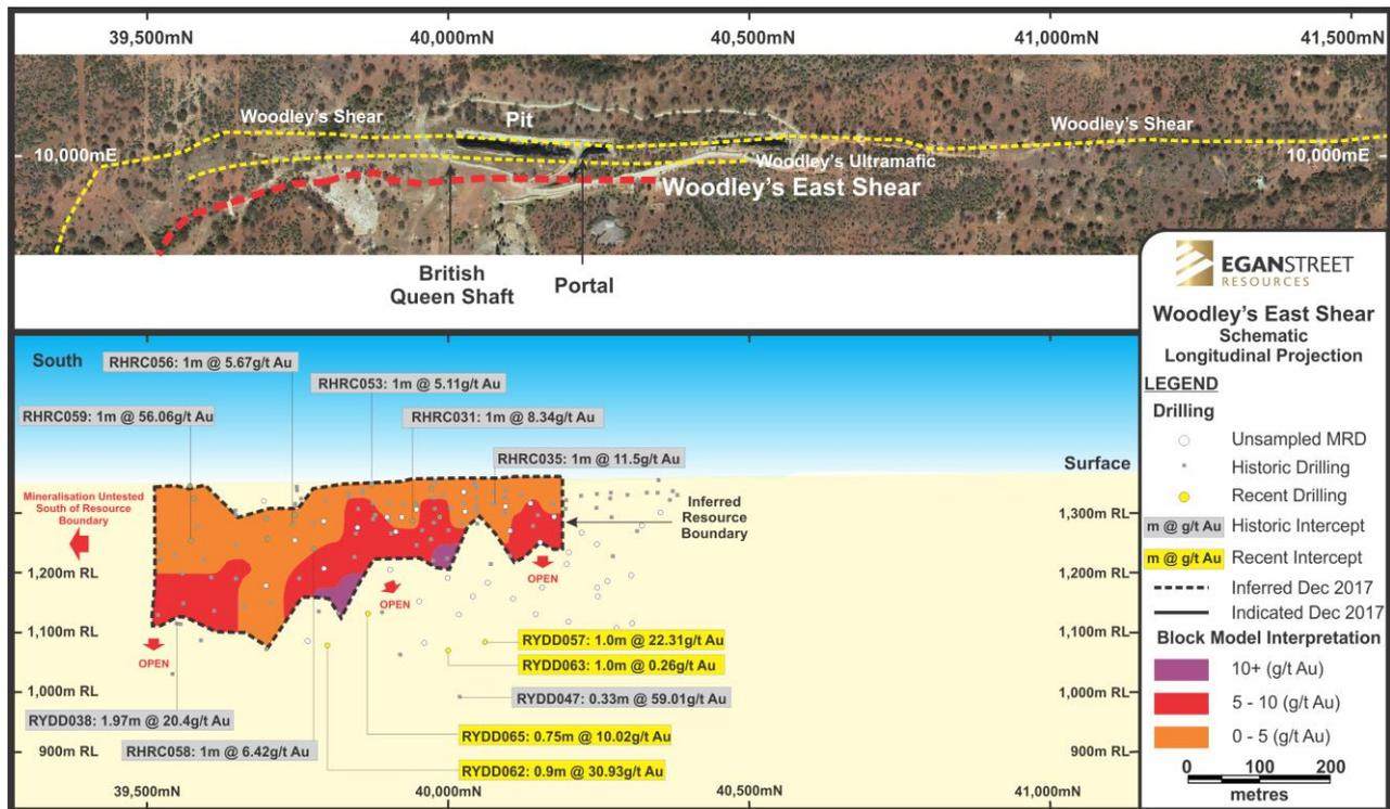
FIGURE 1 – WOODLEY'S SHEAR SHOWING SIGNIFICANT & RECENT INTERSECTIONS
