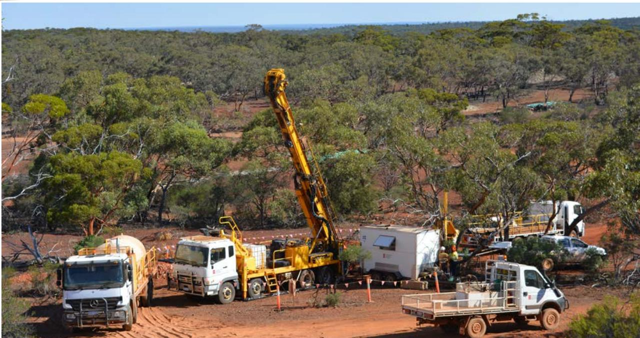
FIGURE 3 – DIAMOND RIG DRILLING AT ROTHSAY
